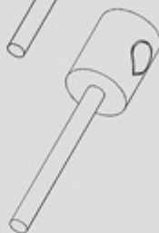
D2: DERAILLEUR CABLE FOR CAMPAGNOLO NIPPLE SIZE: 3.9 x 5 mm
