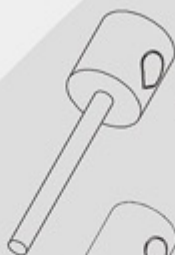
D1: DERAILLEUR CABLE FOR SHIMANO & SRAM NIPPLE SIZE: 4.4 x 4.4 mm
