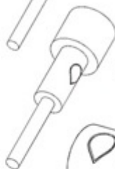
R2: BRAKE CABLE FOR ROAD CAMPAGNOLO NIPPLE SIZE: 5.5 x 11.5 mm
